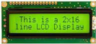
Fig-5 LCD Display
