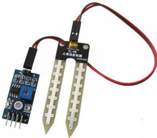
Fig- 2 Soil moisture sensor
